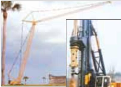
Liebherr Crawler Cranes and Drilling and Pile Driving machines with lift crane capacities to 330 ton and tip heights to 493 feet, duty cycle machines with up to 900 HP engines and line pulls to 88,000 lbs and Drilling and Pile driving machines with up to 900 HP engines and working torque to 295,000 foot pounds and leader lengths to 140 feet.
